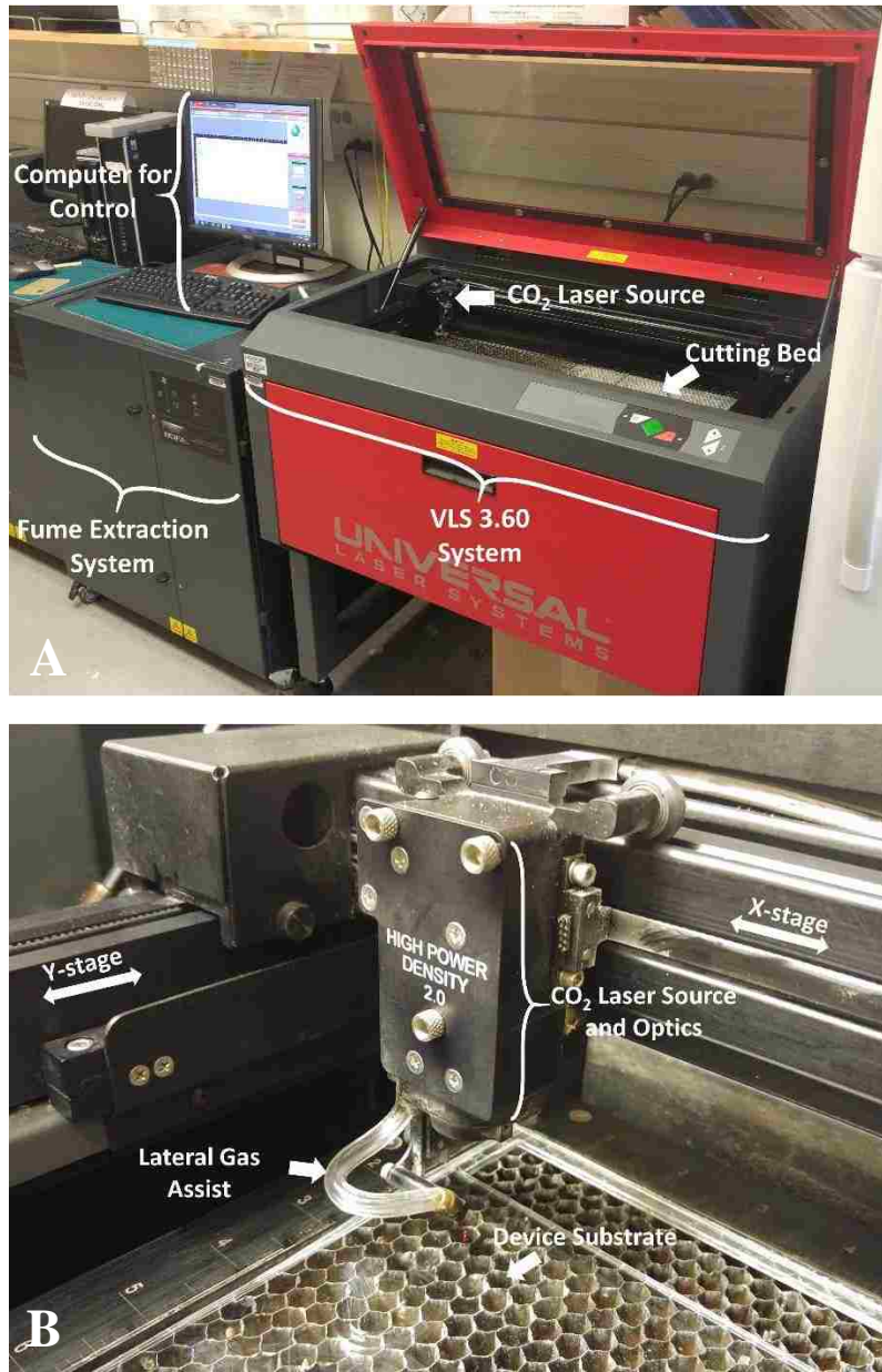
Figure 6: VLS 3.60 laser system. (A) Laser system and peripheral components. (B) Laser source and optics along with lateral gas assist and mechanism of movement across substrate.
