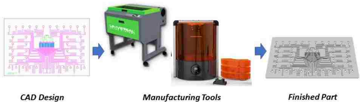
Figure 2: Digital microfluidic manufacturing process flow
